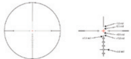
Detail of the AMD reticule, note the circular dots and 1/2-Mil hash marks in between
