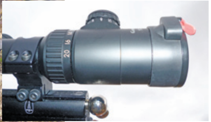
Close up of the eyepell showing magnification ring, reticle illumination dial and Butler Creek flip up caps
